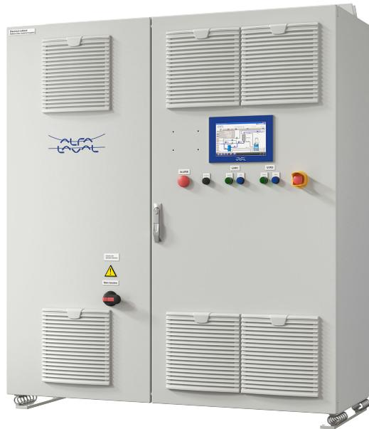
The PureBallast 3 Ultra, electrical cabinet provides power to the UV lamps and can be placed up to 100 m away from the UV reactor. It features a 10" graphical touchscreen interface that is easy and intuitive to use. Operation can be started or stopped with a single touch. The control system can be integrated with onboard automation systems via Modbus, allowing access to all functions through the vessel's Integrated Ship Control System.
