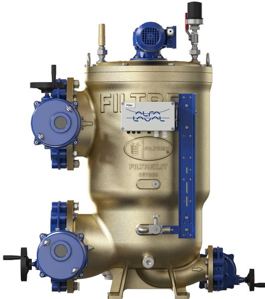
A filter is used during ballasting operations to block the intake of larger organisms and reduce sediment in the ballast water tanks. Bypassed during deballasting, the filter is cleaned via automatic backflushing using a small portion of the system flow. This not only improves backflushing efficiency, but also increases overall filter effectiveness by producing a higher net capacity.
