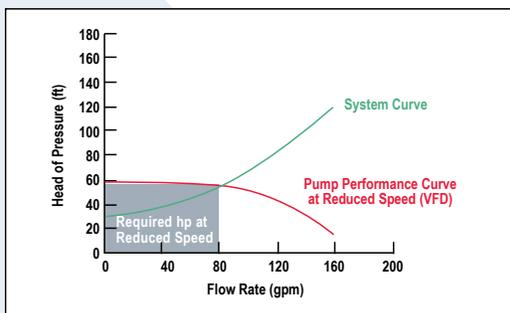
Figure 3. System characteristics using a variable frequency drive
