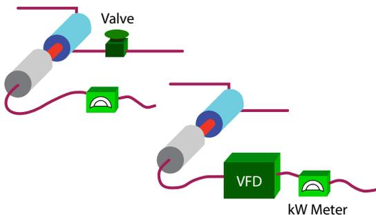
Figure 1. A mechanical throttling device versus a VFD
