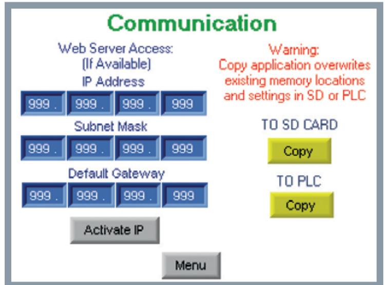
Use the available SD card to transfer information, or connect the system to your network using the built-in Ethernet port. When connected using Ethernet, you are able to view the system performance and operation from any computer or mobile device with web access.
