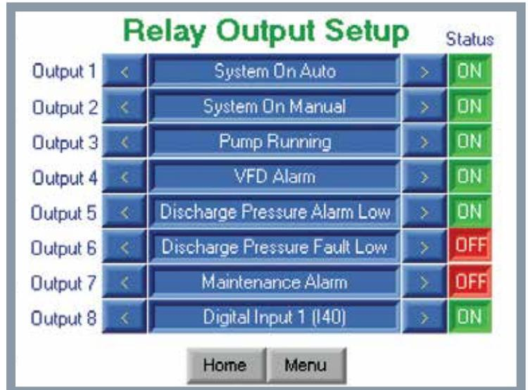
Monitor the system through the use of four standard relays. An additional four relays may be added to the system as an option.
