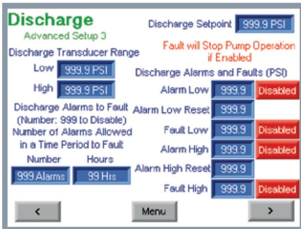
Determine your Alarm and Fault tolerances. Alarms will reset once operating conditions return to normal. Faults will cause the system to stop operating, resulting in operator assistance.
