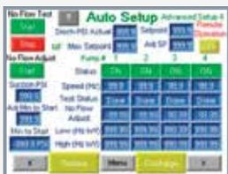
All system adjustments are made on a large 5.7" color touch screen and based on the building's unique profile demands, reducing the need for a technical expert to perform start-ups.
