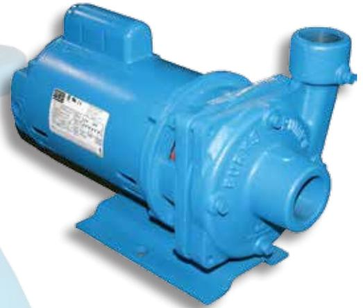
**Series GN Base-Mounted Centrifugal Pumps** are available in 1750 RPM, with capacities to 1100 GPM, heads to 95 feet; and in 3500 RPM with capacities to 950 GPM, heads to 380 feet. The base-mounted pump models are rated for use on inlet pressures to 100 psi, and case working pressures to 200 psi, with suction sizes from 1½" to 5", and discharge sizes from 1¼" to 4".
