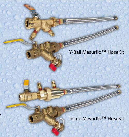
HoseKits are a convenient method of combining the advantages of flow control and a flexible connection. Our kits are supplied with a Mesurflo™Automatic Balancing valve, a non-ported ball valve, two stainless steel braided hoses, and a ball valve with P/T ports. All kits are 100% leak tested before shipping!
