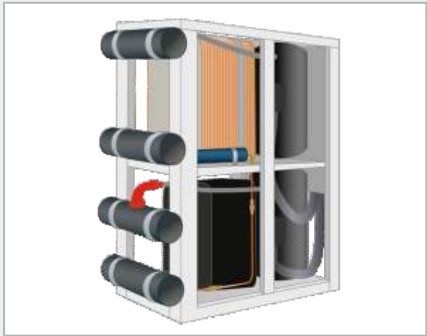
SWEP brazed plate heat exchangers work as evaporators, condensers, or economizers in a range of chiller systems.
