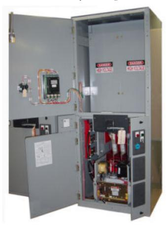
Medium Voltage Switchgear is provided in compartmentalized structures removable circuit breakers, highly insulated bus, and vacuum type draw-out starters. TLC can package these starters with Motor Protection systems to comprehensively protect these pumps providing overcurrent, undercurrent, imbalance, and back spin protection. Additional metering can also be provided to monitor line voltage and motor current.
