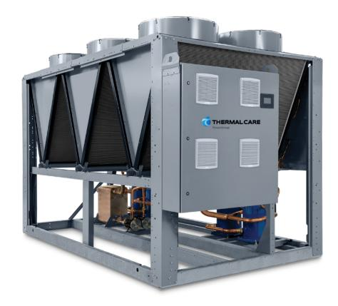
30RC Series Air-Cooled Central Chillers come in an all-inone package and are easy to install, operate and maintain. Available in a capacity range from 130 to 260 tons (457 to 914 kW), using EPA approved low GWP R-454B refrigerant. The 30RC Series features robust scroll compressors, durable construction designed for outdoor installations, and a microprocessor control system for precise operation and
