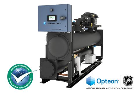
Thermal Care is at the forefront of process cooling technology. TC Series industrial central chillers feature revolutionary, frictionless, magnetic bearing Turbocor compressors for optimal performance and unmatched part load efficiency. The oil-free design eliminates oil management systems, reducing costs and environmental impact while enhancing reliability.
