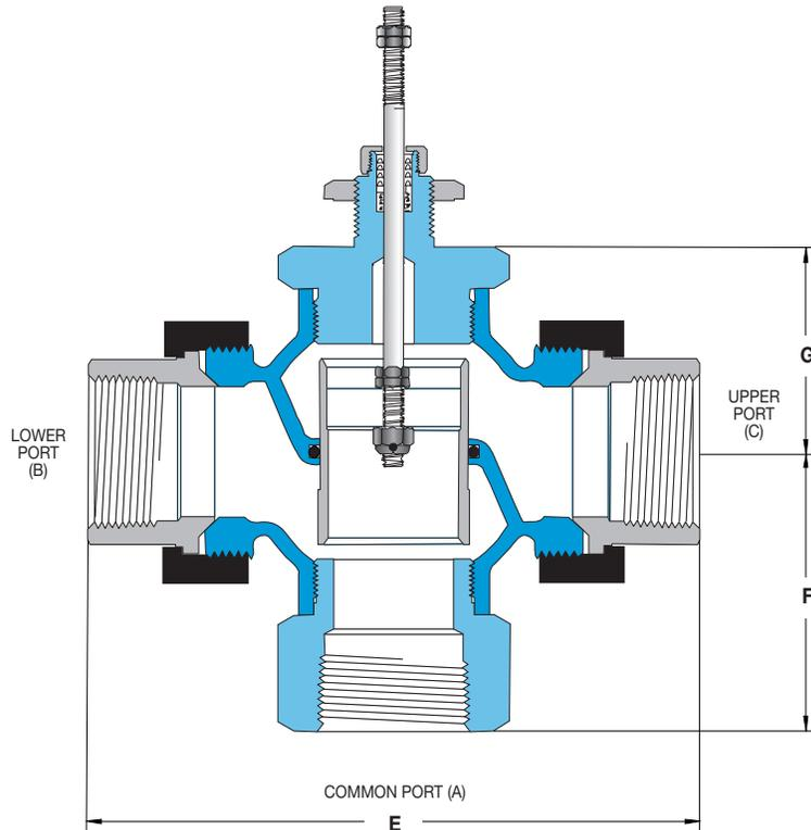
Trerice 3-Way Valves are not designed for use in steam applications. To properly control the mixing of two flows, inlet pressures at ports B and C should be as equal as possible.
