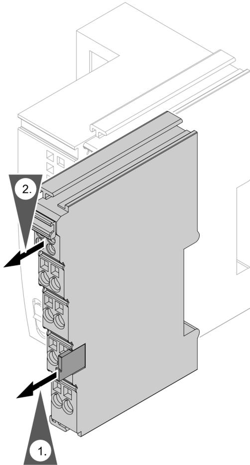
If the gateway or power supply unit need to be removed, e.g. because the device is faulty, proceed as shown in the following diagrams.
