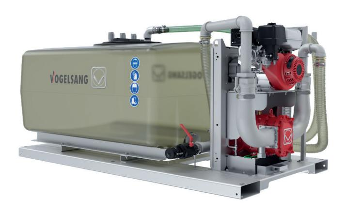
The MobileUnit M Eco WD is a disposal assembly with tank and pump unit for various carrier vehicles. This system enables the emptying of sanitary wastewater collection reservoirs of passenger trains, buses and boats.
