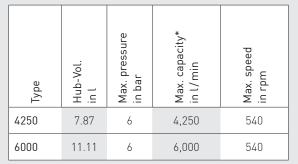
\* Maximum theoretical volume flow. In practice, the capacity is normally lower, depending on pressure difference, medium viscosity, and pump installation. We would be happy to configure the best rotary lobe pump for your application with the help of our computer-assisted dimensioning software.
