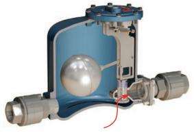
**Steam Trap internal to pump body** will function like a normal float trap discharging condensate as its formed. If condensate backs up, the pumping mechanism will use motive steam pressure to discharge the condensate.
