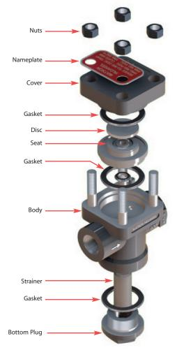
Complete internal working mechanism can be replaced while trap body remains connected in-line
