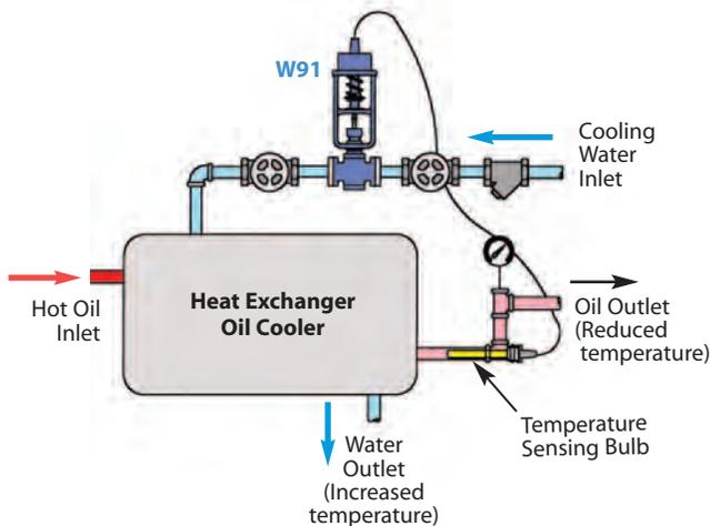
**W91** Cooling valve controlling the flow of water through a heat exchanger to maintain the temperature of oil that is gaining heat by some process. The valve automatically shuts off when not required, greatly reducing cooling water usage. The source of the cooling water may be a well or city water supply and it can be circulated or dumped to drain. A 3-way valve may be used on cold water chiller systems so flow can be diverted from going through the heat exchanger when not required.
