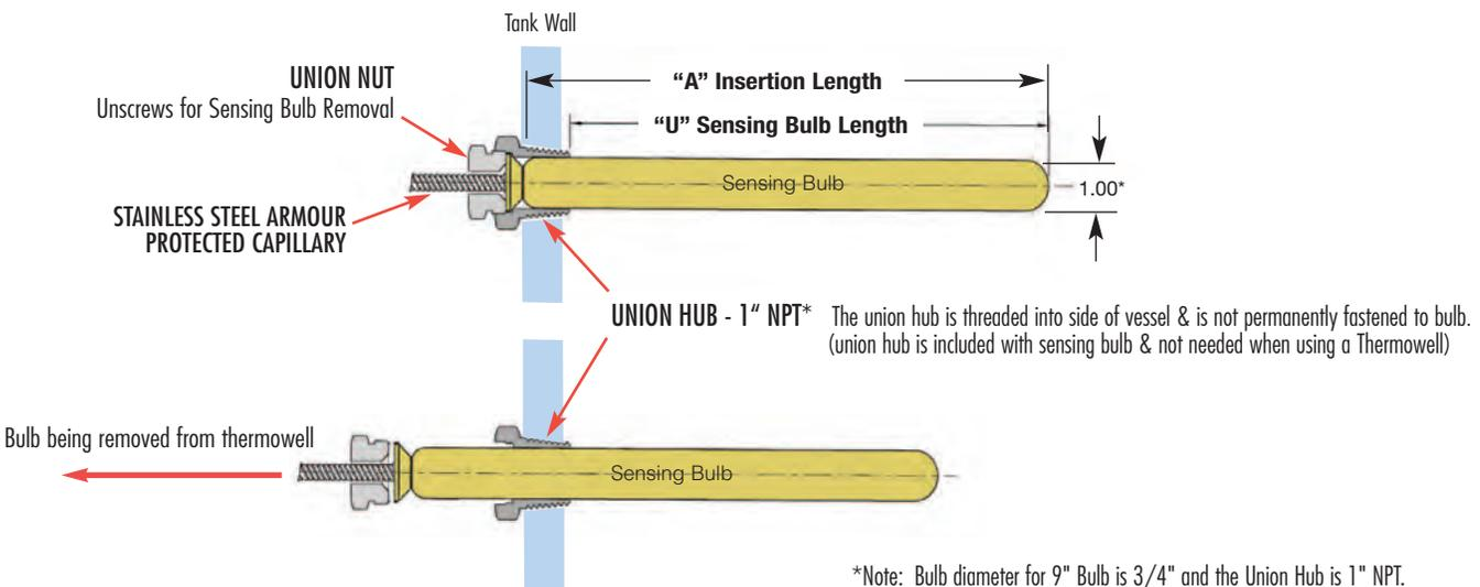
\*Note: Bulb diameter for 9" Bulb is 3/4" and the Union Hub is 1" NPT.
