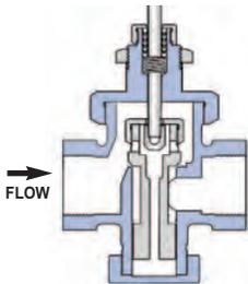
**Normally Open Valves** are used for **HEATING**, so the valve stem closes (**in-to-close**) as the control signal (temperature) increases.
