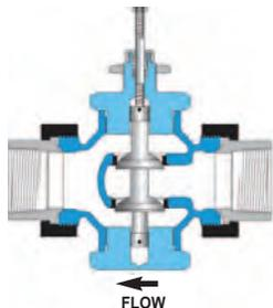
**Normally Closed Valves** are used for **COOLING**, so the valve stem opens (**in-to-open**) as the control signal (temperature) increases.
