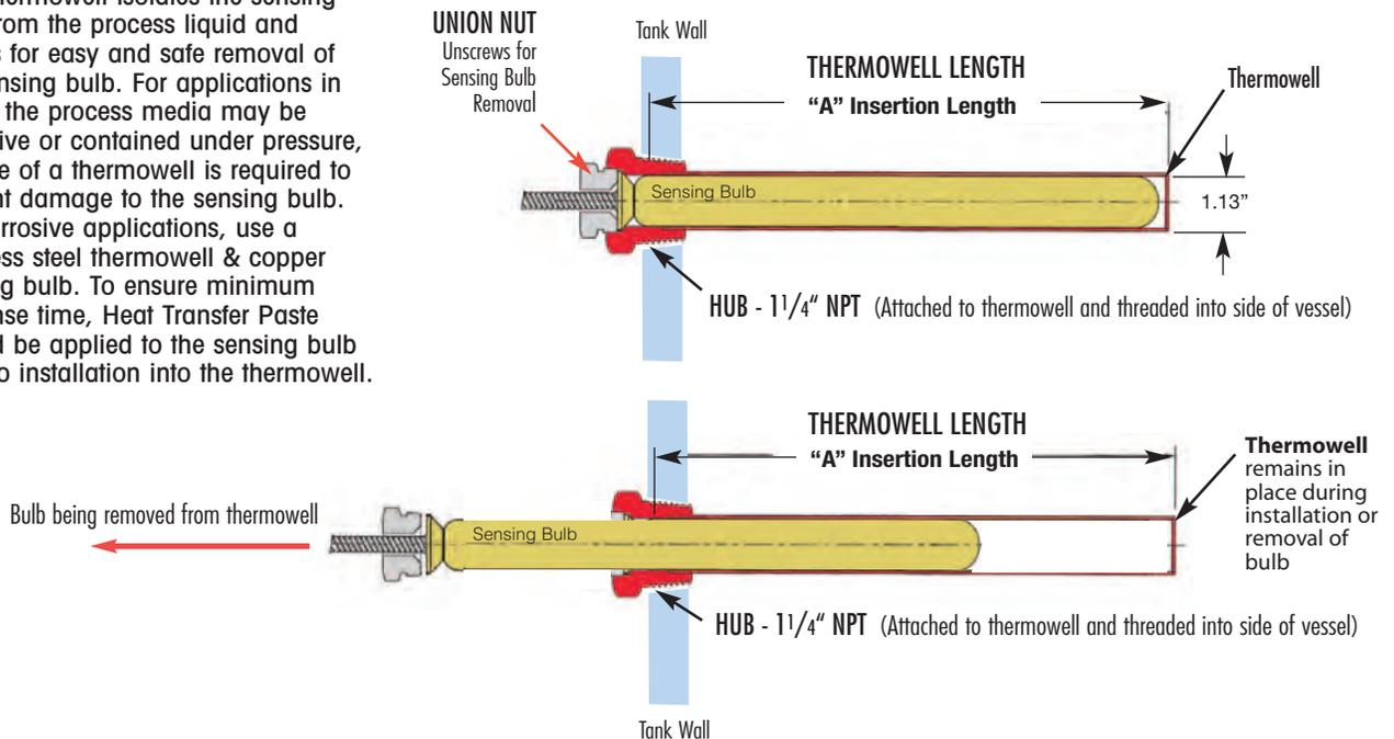
\*Note: Bulb diameter for 9" Bulb is 3/4" and the Union Hub is 1" NPT.
