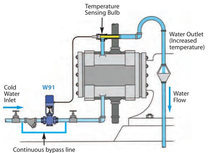
When the Sensing Bulb is mounted remotely from the actual point of Cooling (as shown), the water **MUST** continue to flow so that the sensing bulb can sample the product temperature of the unit being cooled. Without continuous water flow, the temperature control valve will never turn on, causing the unit to overheat. The bypass line provides a minimum continuous flow when temperature set point is achieved and the valve is closed.
