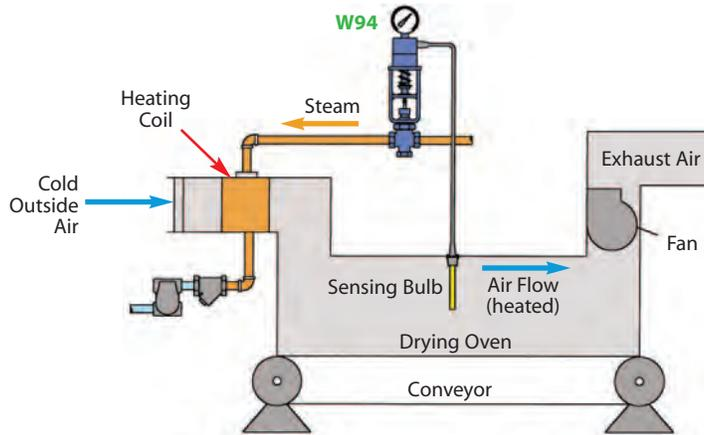
**W94** Valve used to regulate the temperature of the air flow through an air heating duct. The sensing bulb is installed toward the end of the heating duct and will sense the temperature of the air flowing past the heating coils. When air temperature is below the set point, the valve will open to allow more steam through to the coils to heat the air passing through the duct. Once the desired air temperature is achieved, the valve will begin to modulate closed to maintain the air temperature.
