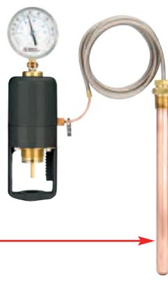
**Model W94 Actuator** is equipped with an integral dial thermometer to indicate sensing bulb temperature. The W94 displays the temperature at the sensing bulb. This allows for easy adjustment of the temperature set-point, as well as continuous monitoring of the application, without the installation of an additional thermometer.
