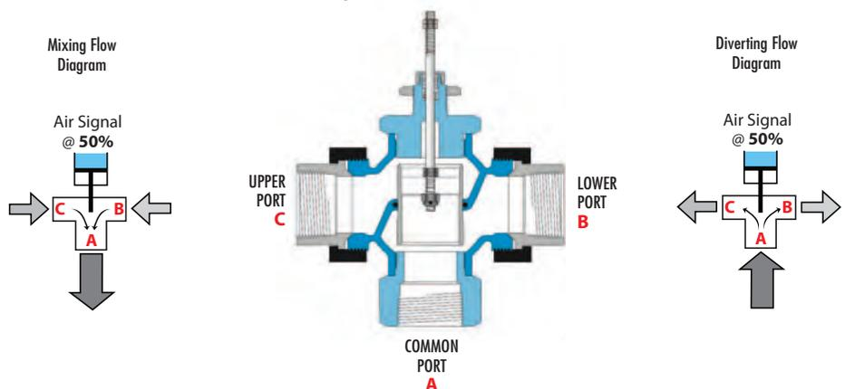
**CAUTION:** 3-Way Valves are not designed for use in steam applications. To properly control the mixing of two flows, inlet pressures at ports B and C should be as equal as possible.
